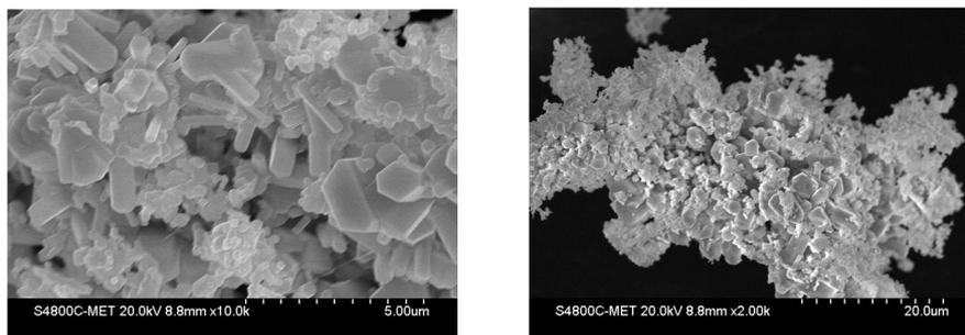
Fig. 2. FESEM images (a) and (b) correspond to heated admixture of PPS and zinc nitrate in molar ratio of 1:1
